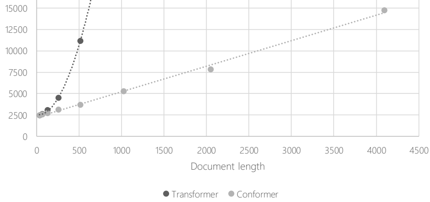
Figure 2: Comparison of peak GPU Memory Usage in MB, across all four GPUs, when employing Transformers vs. Conformers in our proposed architecture. For the Transformer-based model, we only plot till sequence length of 512, because for longer sequences we run out of GPU memory when using Tesla P100s with 16 GB of memory.
