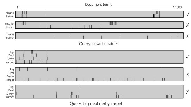
Figure 2: Visualizing patterns of query term matches in documents. Query terms are laid out along the vertical axis, and the document terms along the horizontal axis. The short vertical lines correspond to exact matches between pairs of query and document terms. For both queries, the first document was rated relevant by a human judge and the following two as non-relevant. The query term matches in the relevant documents are observed to be more clustered, and more localized near the beginning of the document.
